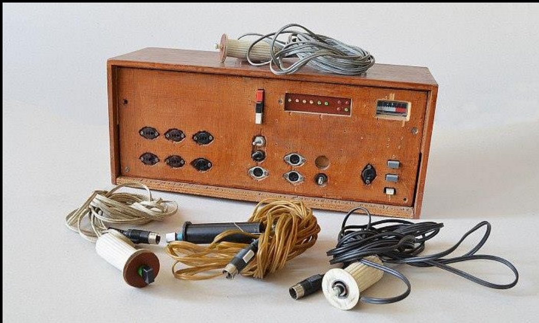
A very heavy reel-to-reel tape recorder for audio recording of the observation time.
